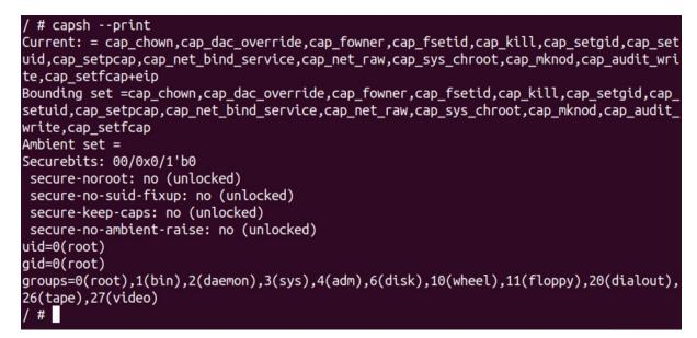
In the preceding image, if we notice the list of capabilities that this container has for this user, there are only a few capabilities that are given to this container by default. This is just a subset of a large number of capabilities that we can have for a root user.
