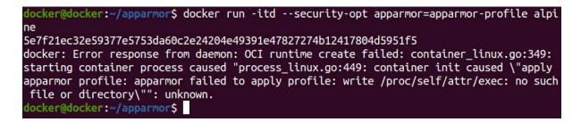
From the preceding image, we can see that the docker run command failed when it tried to load the AppArmor profile. That is because Docker expects to find an AppArmor policy to be loaded and enforced. The AppArmor profile that we are trying to use with the container is not loaded yet. To load it, let us use the following command.
