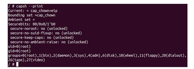
From the preceding image, we can see that there is only one capability available for this container that is chown. This is how we can drop all capabilities apart from the ones that we want in the container and this is how we can make use of capabilities to have granular control on what privileges the root accounts can have.
