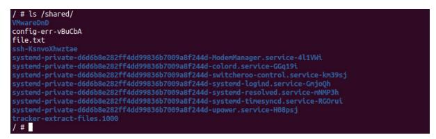
We can see in the preceding image that the entire tmp folder from the host is mounted here. Now let's try to modify the file.txt on the container and see if these changes will take place on the host machine. To do that type the following command on the shell.
