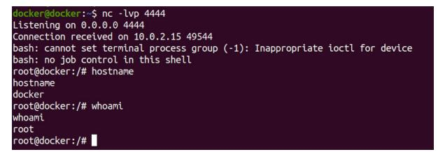
This is how an attacker can escape a container to get root access on the underlying host by abusing CAP SYS MODULE capability.
