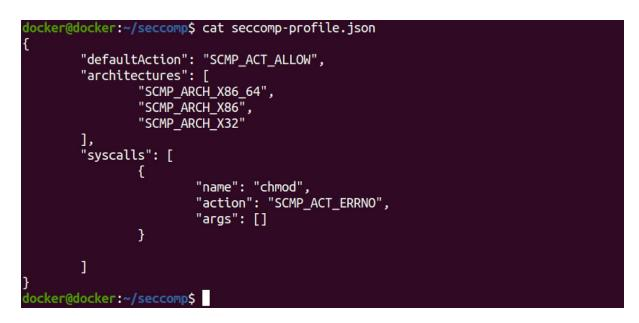
From the preceding image, we can see that the default action is allowed unless we blacklist a specific system call in this list. What this profile does is, it blocks chmod syscall on the container but it will allow anything else. Let us start a new container using this seccomp profile using the following command.
