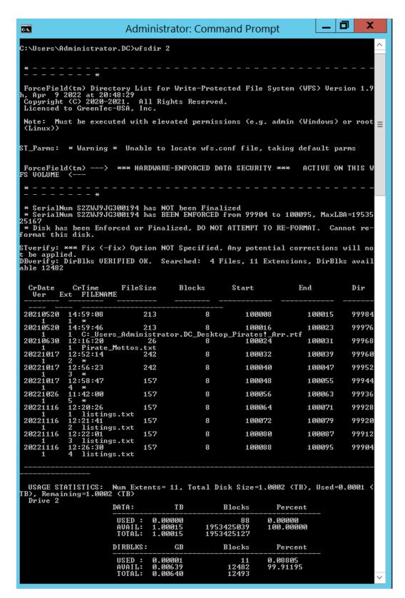
4. Verify that the drives of the Qcor WFS server have been formatted to work with ForceField with wfsdir command line utility that was just installed. The drives may be pre-formatted. Use the
