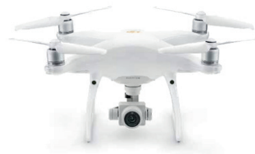
Figure 11: DJI Phantom 3/4 (1380 grams)
