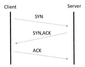
Figure 4-1. TCP Three-Way Handshake
